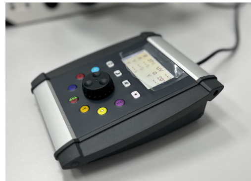
The Viluma 5/7 light control console offers flexible switching across LED wavelengths with precise intensity adjustment.
